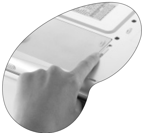
2. Slide the battery retainer to the open position.
